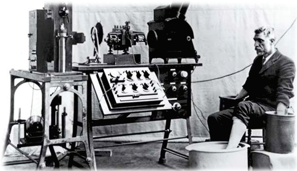
Figure 2. Professor Willem Einthoven invented the first practical ECG device, the string galvanometer, in 1903. The weight was 270 kilograms and it required five technicians to be operated. The person's arms and feet were dipped in salt solutions while the strength and rate of the heartbeat were registered on the chest. Einthoven was awarded the Nobel Prize in physiology and medicine in 1924, "for the discovery of the mechanism of the electrocardiogram". Photo: Google pics. FPG/Hulton Archive/ Getty Images. http://www.nobelprize.org/nobel_prizes/medicine/laureates/1924/einthoven-bio.html
