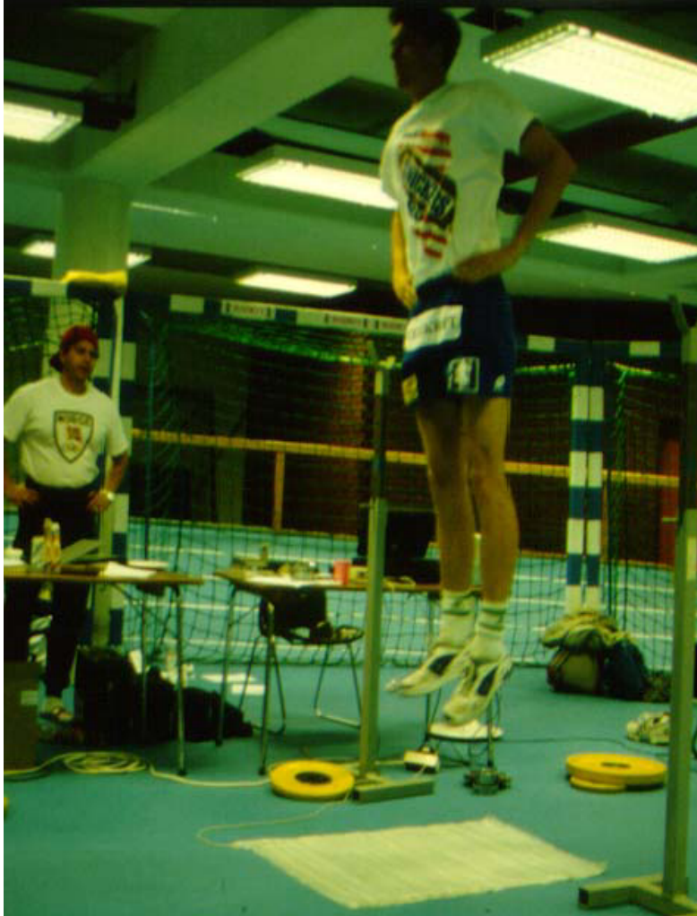
Figure 2. Illustration of the experimental setup for the jump tests. During all tests the players jumped on a contact mat connected to a computer, making it possible to compute jumping height (Bosco et al. 1983).
